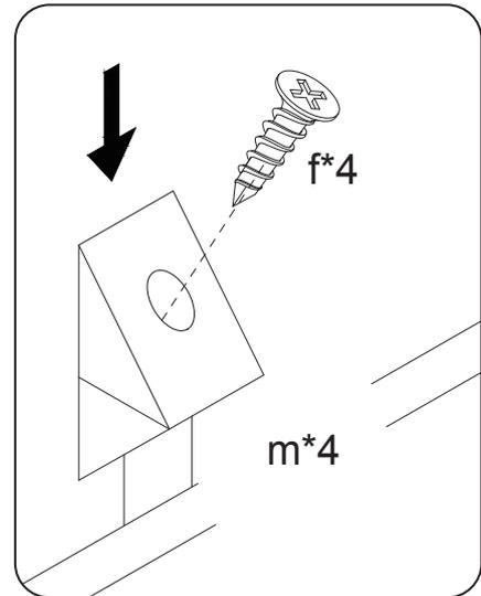
Push x4 (m) into the grooves as shown then fix with screw (f).
